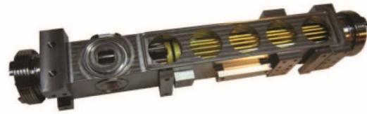
Deep Space Atomic Clock mercury ion trap housing with electric field trapping rods seen in the cutouts. This is where Deep Space Atomic Clock interrogates and measures the mercury ion resonance that is used to discipline a quartz crystal clock.
