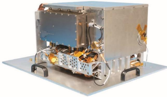
The Deep Space Atomic Clock Demonstration Unit (shown mounted on a plate for easy transportation).
